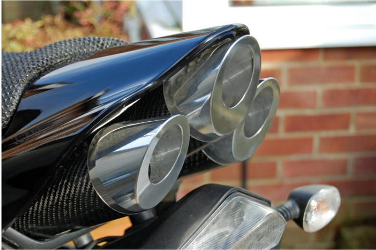
Whilst someone holds the silencers in place, carefully re-mount the light-mounting bracket. You will find that the two outer silencers are held firmly against this bracket and you should carefully ease it in to place so it supports the silencers without damaging them. This is supposed to be a tight fit so that the silencers cannot move at all.
